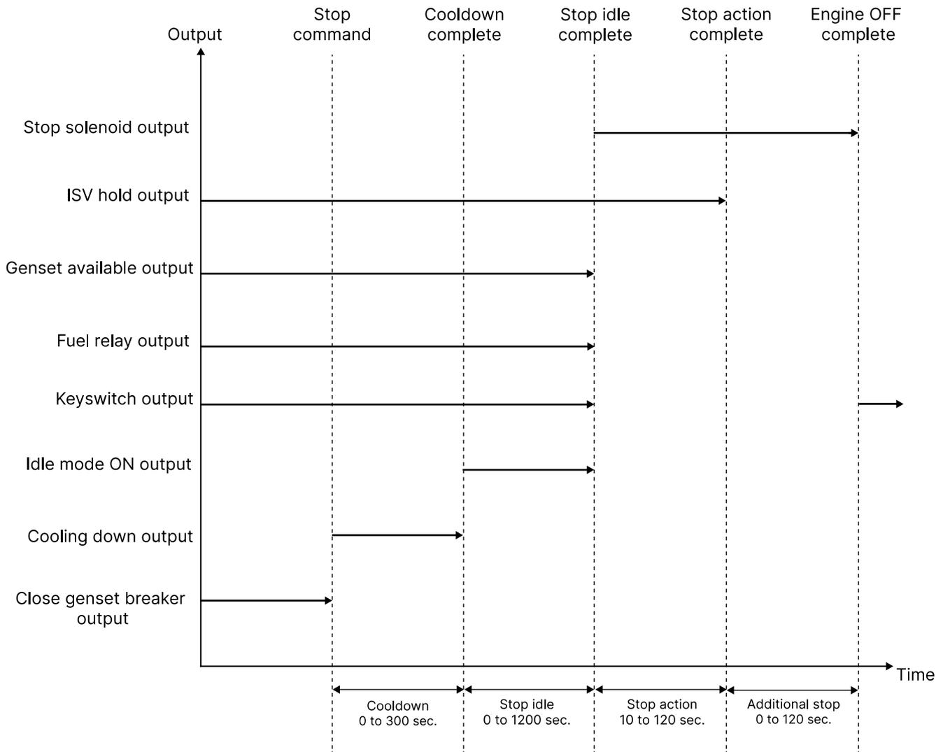
The stop sequence is activated if a stop command is given. The stop sequence includes the cooling down time if the stop is a normal or controlled stop.
