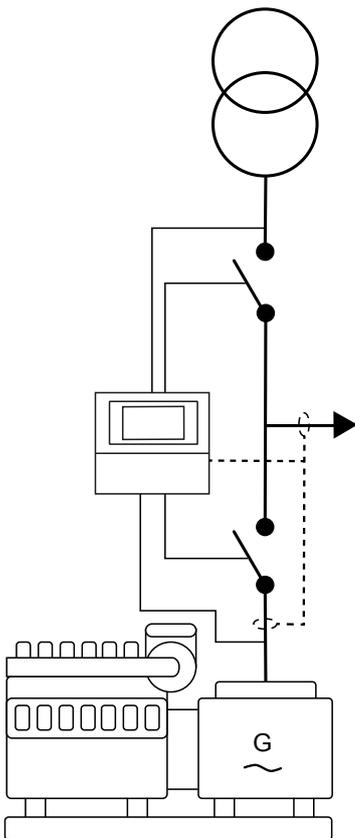
**NOTE** You can place the CT on the line from the genset or on the load side.
