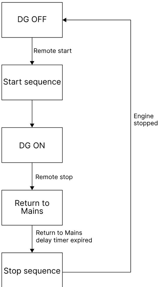
To configure the remote start/stop inputs, go to *Digital Inputs* in the smart connect software and select the source as *Remote Start/Stop*. You cannot use remote start/stop when mains monitoring is enabled. Go to *Mains > Configuration* and make sure the box next to *Mains Monitoring* is not ticked.
