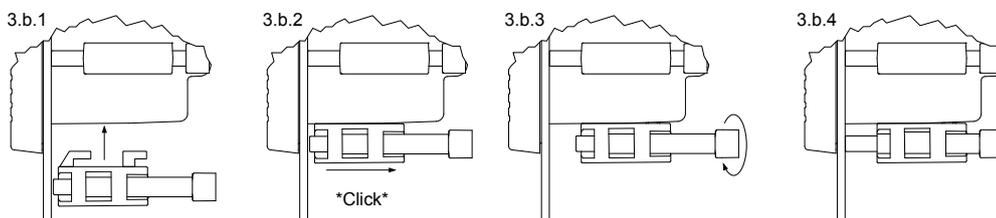
3. Tighten the screw clamps to 0.19 Nm. Do not tighten the clamps to more than 0.19 Nm.
