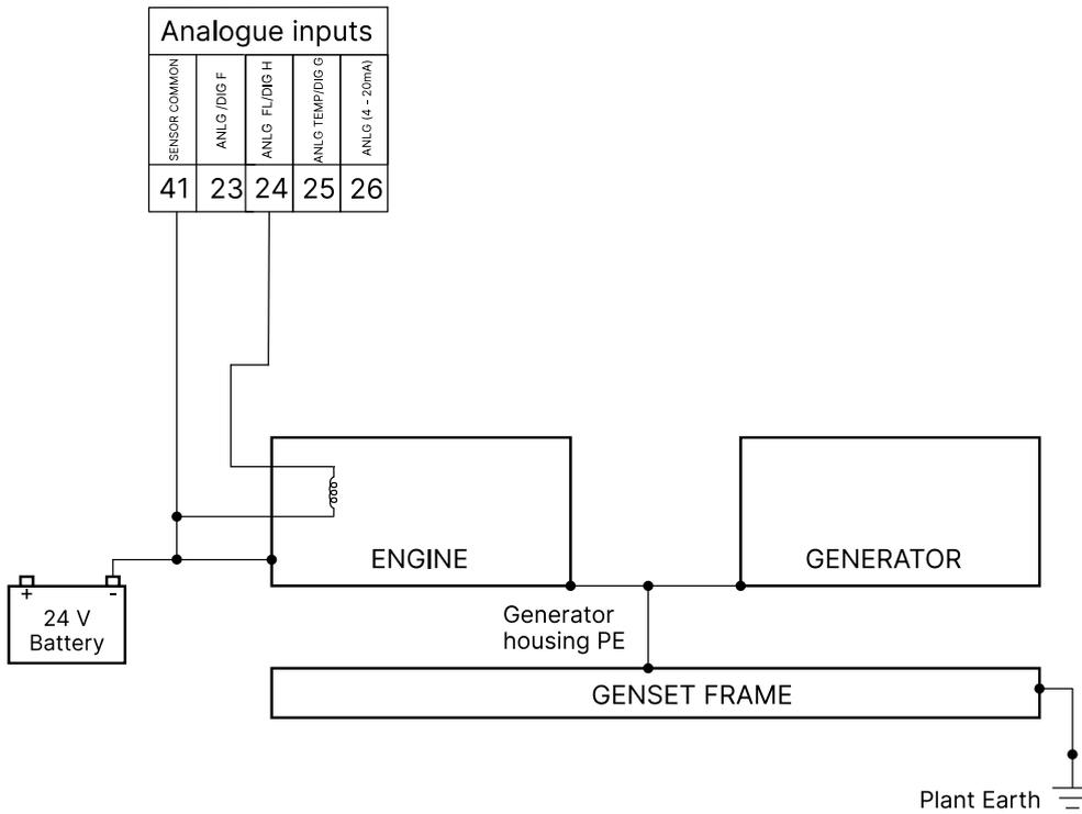
Wiring for the sensor common point (SCP) for analogue input 2 (terminal 24) when you use it as *Fuel level sensor* with reference to *Battery Negative*.
