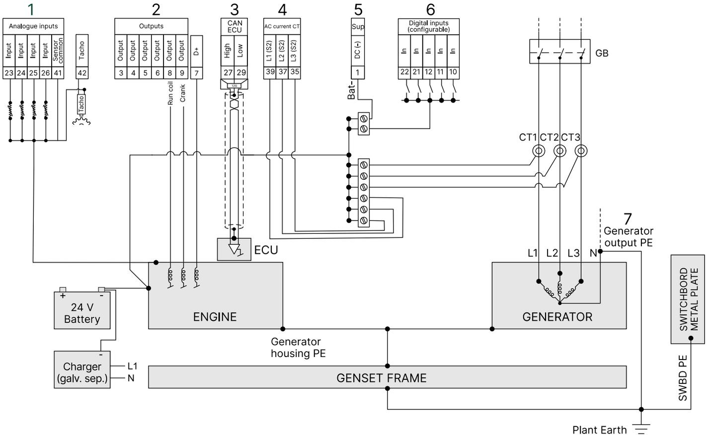
1. Terminal 41 (sensor common point) must be connected to a solidly grounded point on the engine, for example the engine frame. The potential difference to terminal 1 (BAT-) must be less than  $\pm 0.5$  V.
