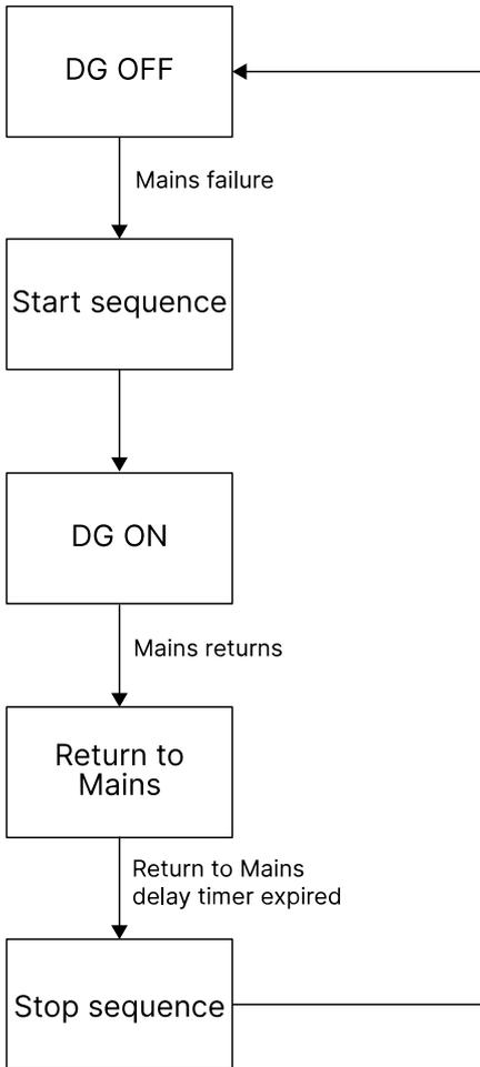
If there is a mains failure, the SGC controller can automatically start the genset and switch to generator supply (see the flowchart above). The controller does this if the mains continues to fail after the *Mains detect delay* timer has expired.
