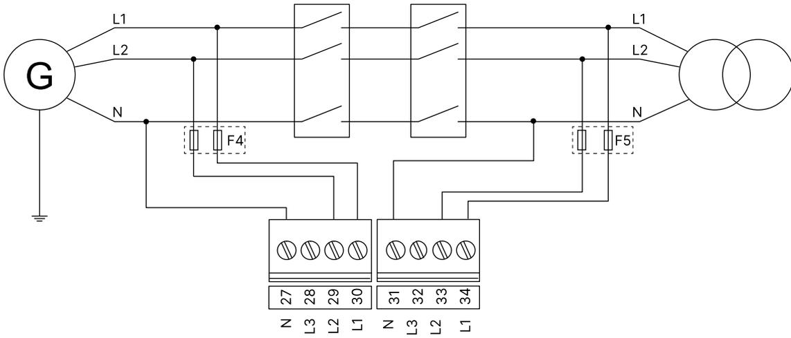
**Two-phase application L1/L3 (3 wires)**
