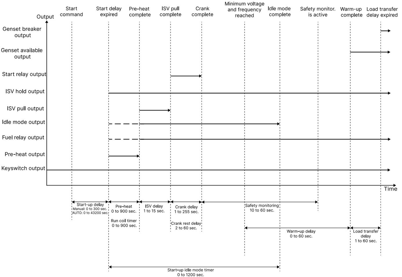
Configure the run coil timer to activate the fuel relay output and the idle mode output before pre-heat is completed.
