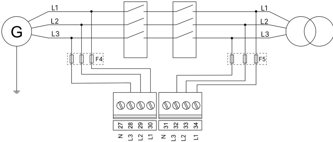
**Two-phase application L1/L2 (3 wires)**
