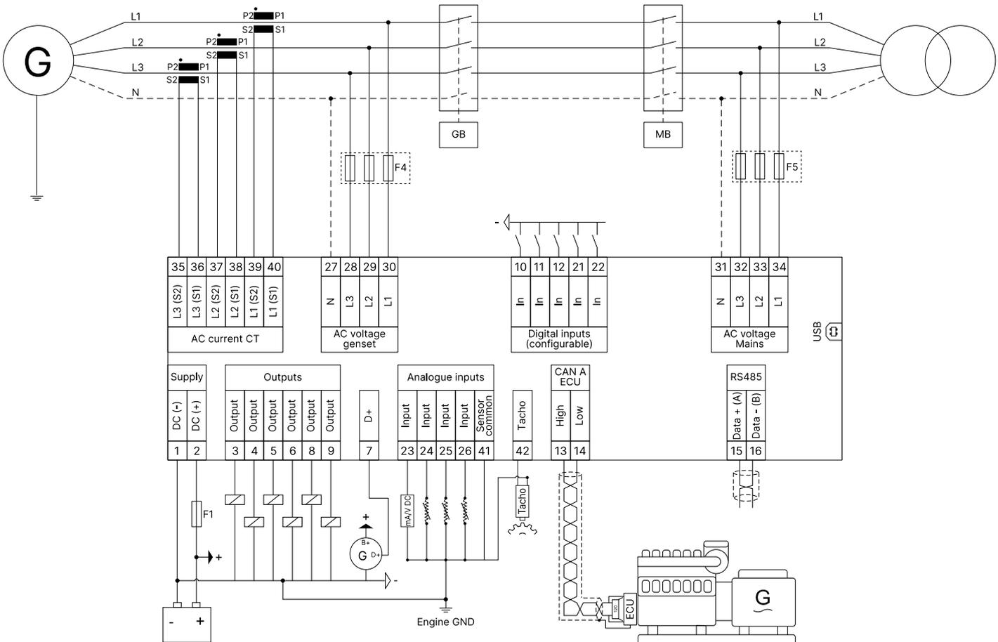
**NOTE** The wiring diagram is only an example. Use the wiring diagram for the specific application during installation.
