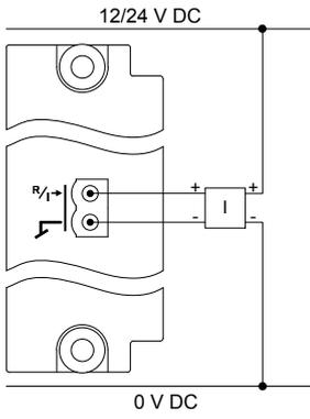
**Figure 4.65** Connection of a passive transducer
