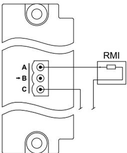
**Figure 4.40** Connection of a 2-wire resistance measurement input (RMI)
