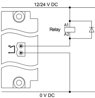
Install a freewheeling diode (
