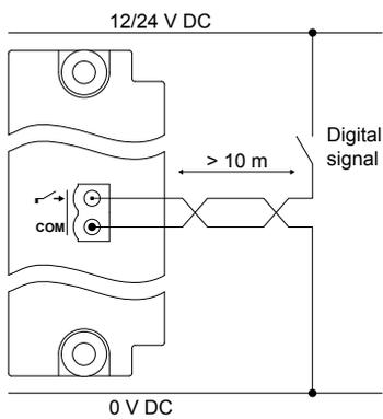
**Figure 4.13** Example: Shielded wire for compliance with EN60255-26
