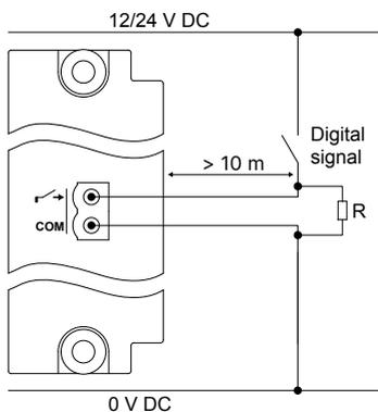
**Figure 4.49** Example: Twisted wire for compliance with EN60255-26
