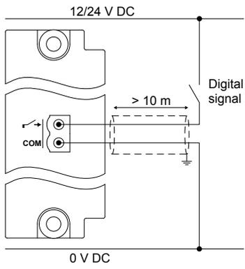
**Figure 4.14** Example: Closed contact for compliance with EN60255-26
