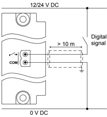
**Figure 4.63** Example: Closed contact for compliance with EN60255-26
