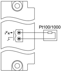
**Figure 4.28** Connection of a 3-wire Pt100/1000 sensor
