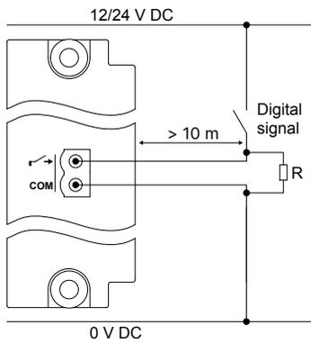
**Figure 4.20** Example: Twisted wire for compliance with EN60255-26
