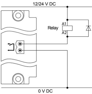
Install a freewheeling diode (
