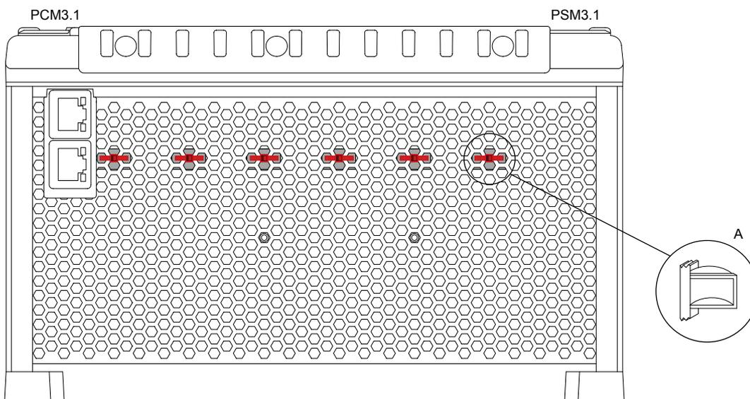
**Figure 3.2** Cable tie slot positions by red cable ties (Slot detail A)
