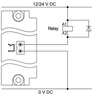
Install a freewheeling diode (
