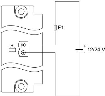
**Figure 4.2** Incorrect wiring of the power supply
