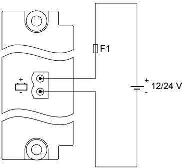
**Figure 4.53** Incorrect wiring of the power supply
