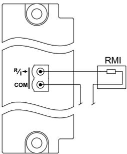
**Figure 4.70** Connection of a 2-wire resistance measurement input (RMI)
