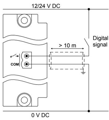
**Figure 4.51** Example: Closed contact for compliance with EN60255-26
