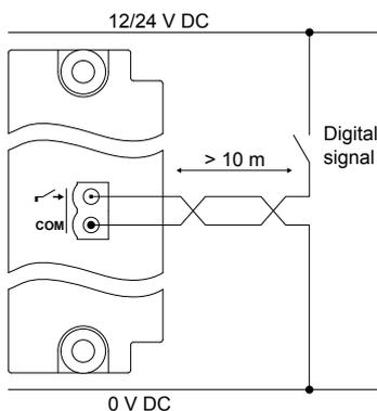
**Figure 4.62** Example: Shielded wire for compliance with EN60255-26
