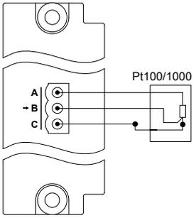
**Figure 4.38** Connection of a 4-wire Pt100/1000 sensor
