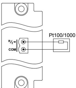
**Figure 4.67** Connection of a 3-wire Pt100/1000 sensor
