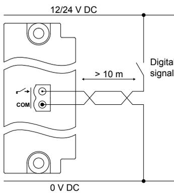
**Figure 4.21** Example: Shielded wire for compliance with EN60255-26
