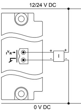
**Figure 4.26** Connection of a passive transducer
