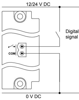
**Figure 4.57** Example: Digital input wiring (common = 12 or 24 V)
