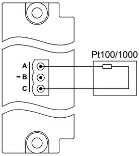
**Figure 4.37** Connection of a 3-wire Pt100/1000 sensor
